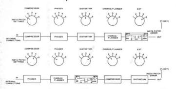
Since only one effect can occupy one place at a time in the series chain, if more than one of the INSTA-PATCH selectors are turned to the same number, the chain is broken and there will be no output from the UE-400. In this case, the INSTA-PATCH ERROR indicator will signal the incorrect condition by blinking on and off. A quick glance at the INSTA-PATCH selectors reveals which one should be turned to a new position to restore the series chain.
